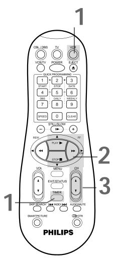
Press the Number 1/START + or Number 4/STARTbutton to set the recording's start time. Every time you press a button, the start time changes in one-minute increments. If you press and hold a button, the start time changes in 30-minute increments.
