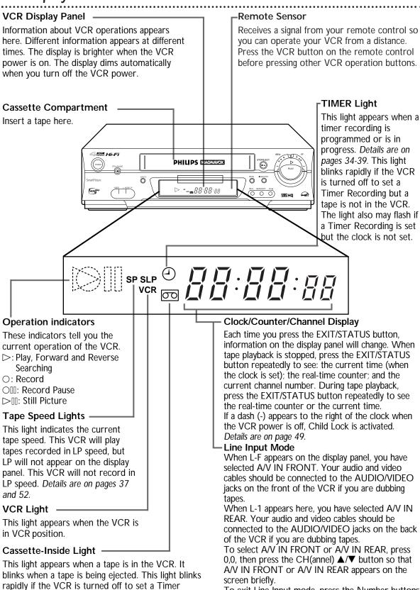
To exit Line Input mode, press the Number buttons or the CH(annel) **△**/**▼** button to select another channel.
