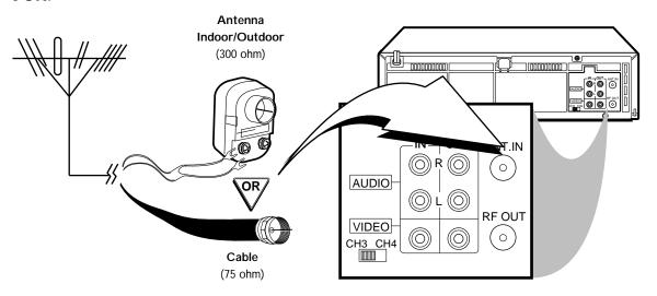
Connect the RF coaxial cable (supplied) to the RF OUT Jack on the back of the VCR and to the ANTENNA IN Jack on the TV. (You may use either a snap-on type or screw-on type of coaxial cable, whichever you prefer. A snap-on type is supplied.)
