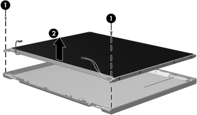
*Removing the LCD Panel*
