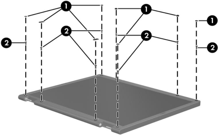
*Removing the Display Bezel Screw Covers and Screws*
