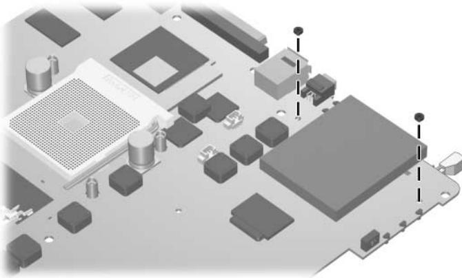
*Removing the PC Card Assembly Screws*
