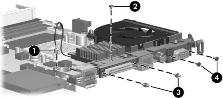
*Removing the Fan Assembly Screws*
