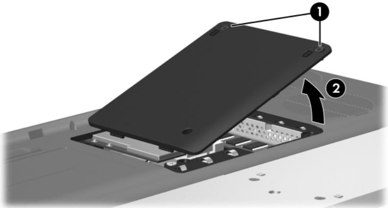
*Removing the Memory/Mini PCI Module Compartment Cover*
