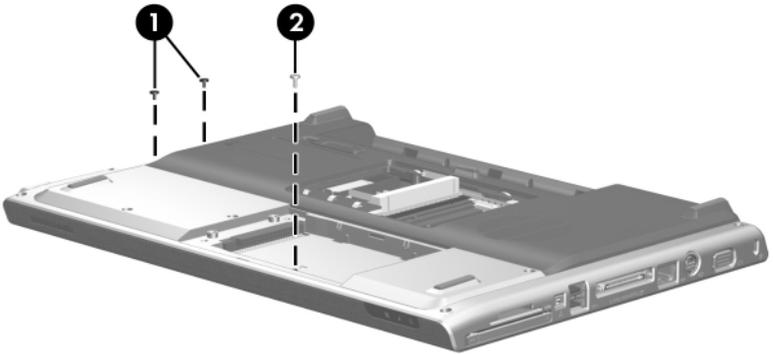
*Removing the Top Cover Screws, Part 1*
