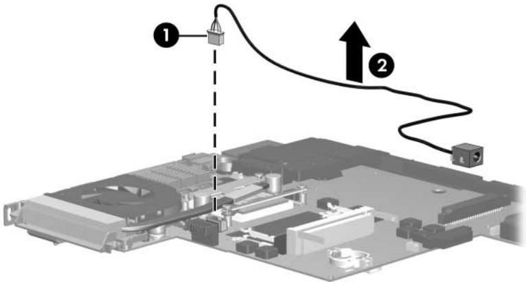
*Removing the Power Connector Cable*
