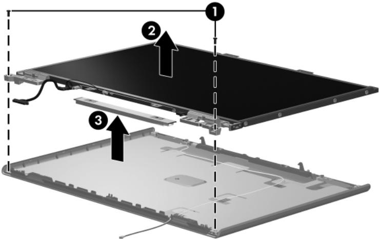
*Removing the Display Panel and Inverter Board*
