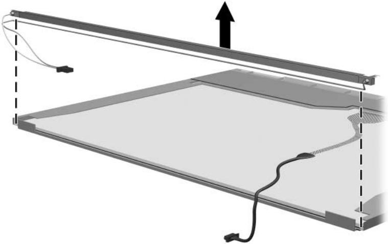
*Removing the Backlight Frame*
