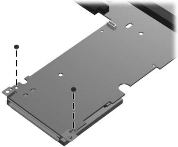
*Removing the ExpressCard Assembly Screws*
