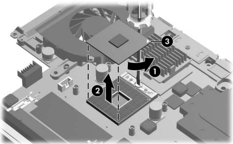
*Removing the Processor from a Socket with a Locking Screw*
