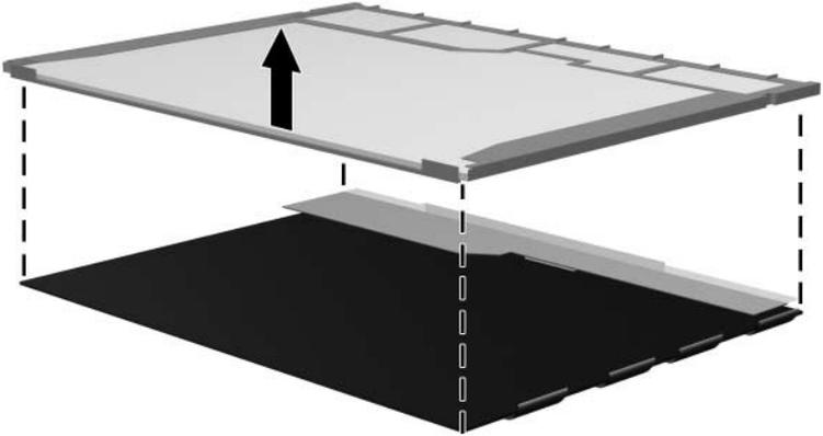
*Removing the LCD Panel*
