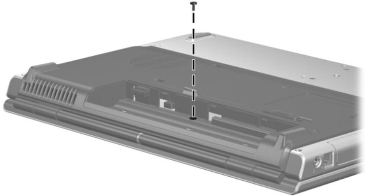
*Removing the Keyboard Frame Screw*
