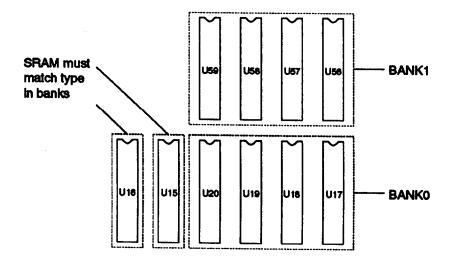
8KB or 32KB SRAM chips can be installed. Bank 0 must be filled before Bank 1. The SRAM type used for RAM in locations U15 and U16 must match the type installed in the banks. The table below shows the possible configurations.
