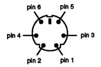
Although the keyboard and mouse connectors are physically identical, they cannot be used interchangeably.
