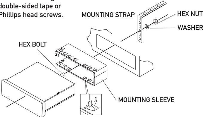
TYPICAL FRONT-LOAD DIN MOUNTING METHOD
