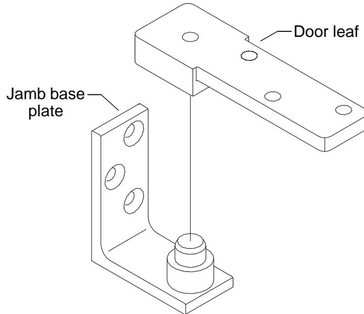
1. Prepare and mortise bottom of door and floor to receive pivot set. Determine pivot location using dimensions on reverse side. Depth of mortise in the bottom of door will determine clearance. **Be sure to properly locate and mark pivot center point of the base plate.**
