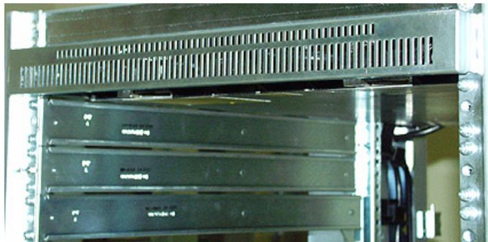
10. Plug one of the supplied power cords into each of the switch's two power receptacles.
