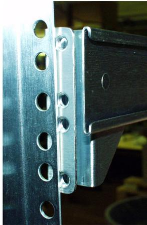
8. Secure the rail to a round-hole rear channel with two M5 x 12 mm screws (see the table on page 3), or secure the rail to a square-hole rear channel with two square-hole washers and M5 x 16 mm screws (see the table on page 3). Leave the screws finger-tight, and tighten them after the switch is installed. See the figure below.
