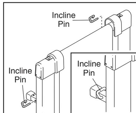
sure that the incline pin is in the “locked” position shown in the inset drawing. Adjust the other incline leg in the same way. **CAUTION: Before using the treadmill, make sure that both incline legs are at the same height and that both incline pins are fully inserted from the direction shown. Do not use the treadmill with the incline pins removed.**
