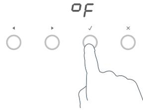
5 Press the right scroll ▶ button to scroll through the options for that particular setting. Refer to the table below.
