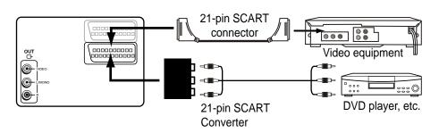
**Note:** If the equipment you want to connect is not equipped with 21-pin Scart, you can connect it by using the **21-pin Scart Convertor** (supplied) as illustrated above.
