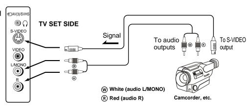
Note: The S-VIDEO input terminal has priority over AV3 VIDEO terminal. To use equipment connected to AV3 VIDEO terminal, disconnect any plug from the S-VIDEO terminal.
