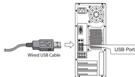
3. Turn On your computer and your operating system will detect the device automatically. This device is plug and play, no driver required.
