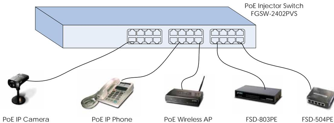
Getting the power from central POE injector, the FSD-504PE shall works without fear of remote power breakdown. As soon as the local PCs also installed with UPS, it shall guarantee the true un-interrupted network accessing.
