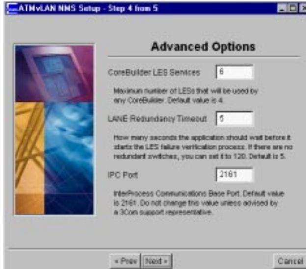
**Figure 1-36** NMS Setup Step 4 Advanced Options
