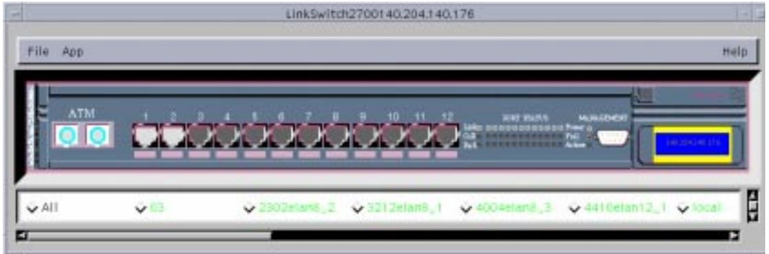
**Figure 5-4** SuperStack II Switch 2700 Front Panel Display
