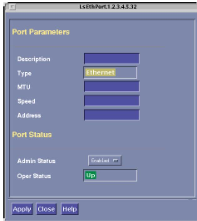
**Figure 4-15** The LsEthPort Parameters Configuration Assistant
