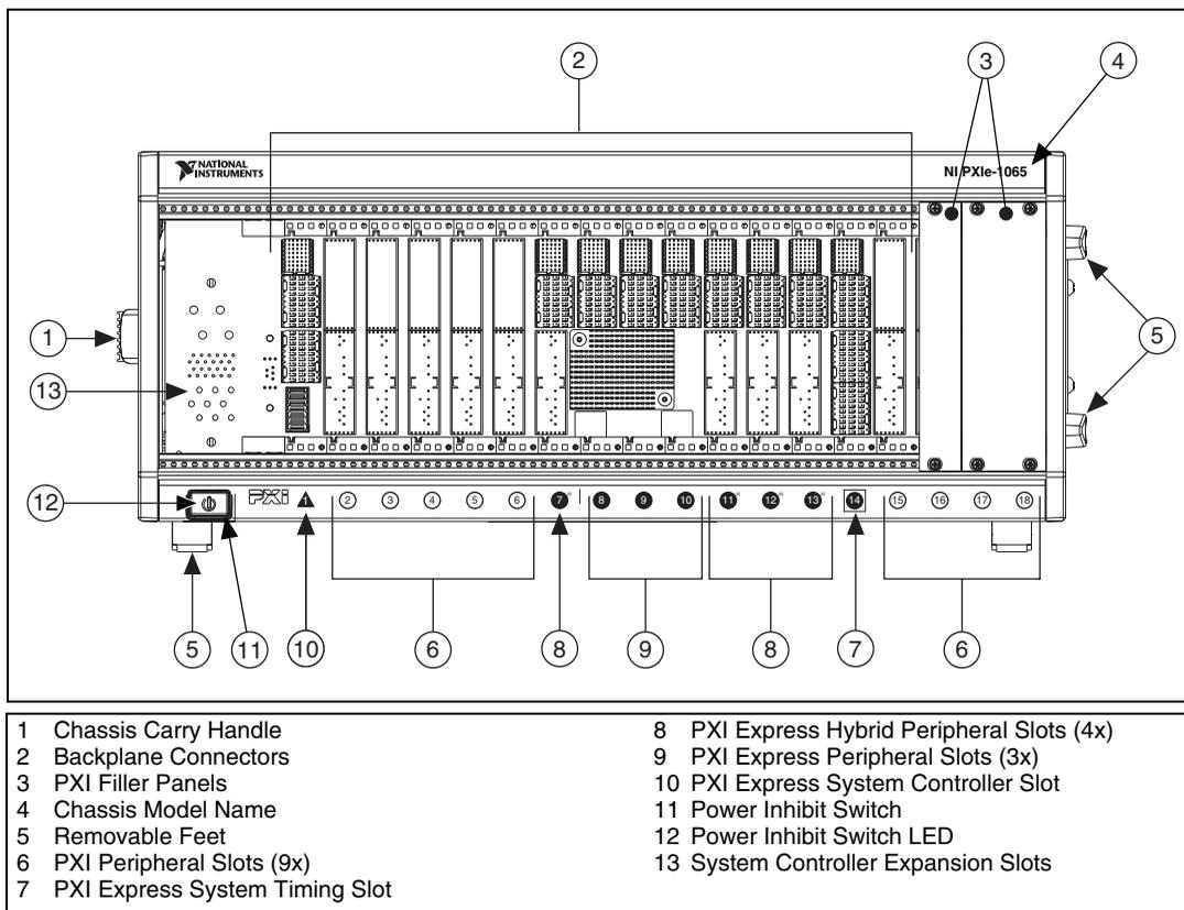
**Figure 1-1.** Front View of the NI PXIe-1065 Chassis
