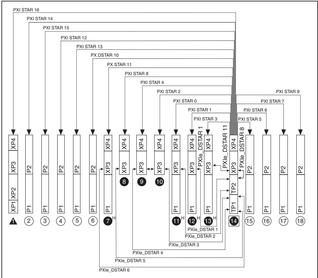
**Figure 1-3.** PXIe\_DSTAR and PXI Star Connectivity Diagram
