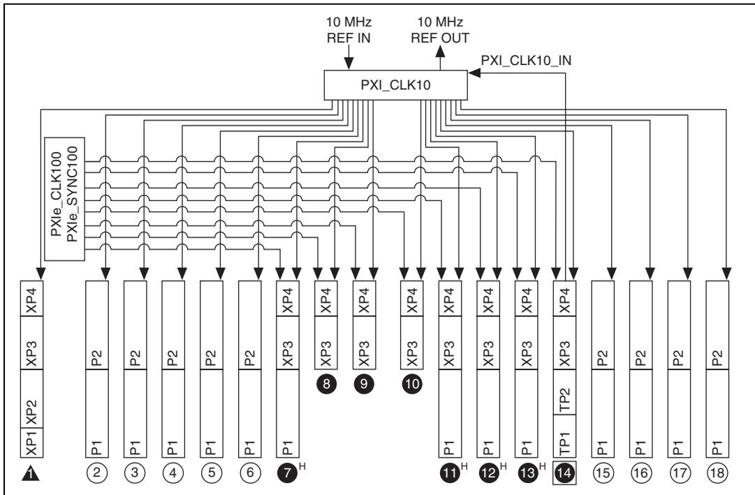
**Figure 1-5.** Distribution of PXI\_CLK10, PXIe\_CLK100, and PXIe\_SYNC100
