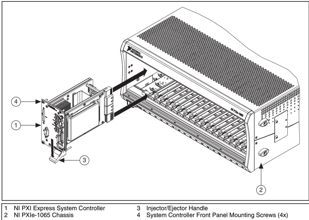
**Figure 2-3.** Installing a PXIe System Controller
