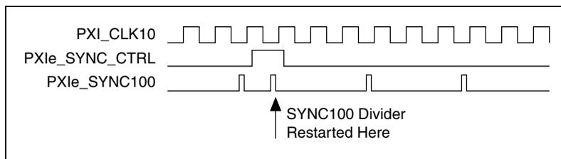
**Figure 1-7.** PXle\_SYNC100 at 3.33 MHz Using PXle\_SYNC\_CTRL as Restart
