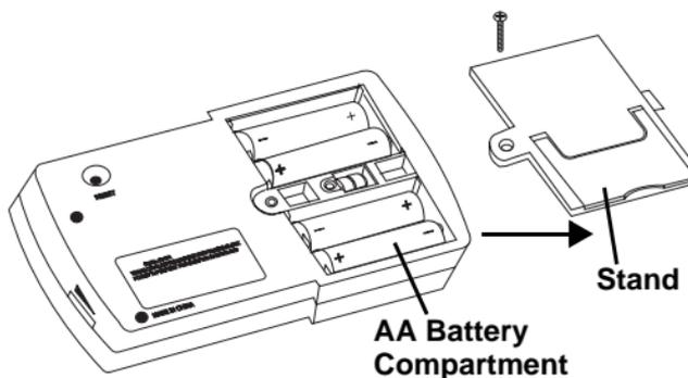
1. Use a Phillips screwdriver to remove the screw from the battery compartment cover, then lift the cover to remove it.
