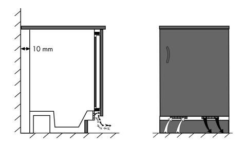
To avoid any loss in performance, air suction channels should not be obstructed. (140 cm2)
