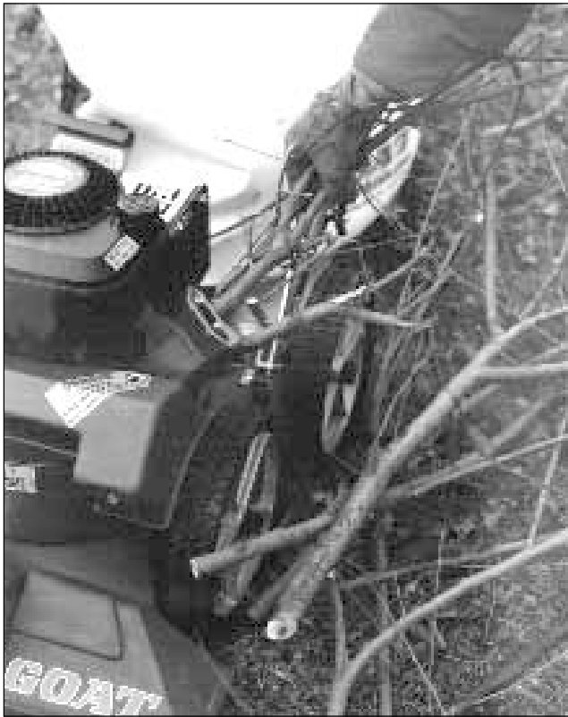
(fig. 2) Note: Dry wood is harder to chip than green wood.
