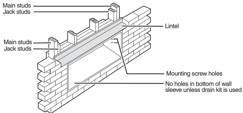
NOTE: Construct wall opening to comply with all applicable building codes.
