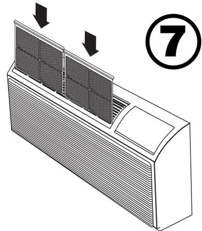
To remove the front cover, remove the thumbscrews at the bottom back corners of the cover (or sides). Pull the bottom end forward and lift it up to clear the L bracket across the top of the chassis.
