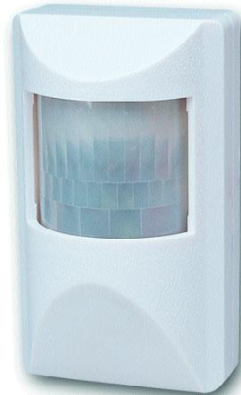
Our 1/3" B/W CCD camera is encased in a white PIR housing. It has a .5 lux sensitivity with 420 line resolution. It features a 3.6mm wide angle pinhole lens and built-in electronic shutter. A 12V DC power supply is included. A color version of this camera can be found under model number VL-565PIR and VL-572PIR (with working PIR). A fully adjustable wall/ceiling mount is included with this unit.
