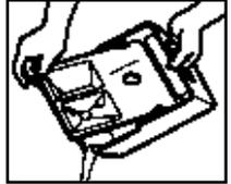
4. Hold water tank by handle and carefully push tank straight into opening in side of unit. Push in until tank is flush with housing.
