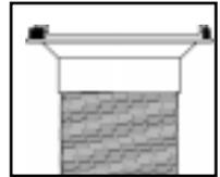
3. Hold connector flange at an angle to the exhaust vent. Press foam gasket on left side of flange against left edge of exhaust vent opening. Slide connector to the left while allowing larger clip to fit behind left side of vent opening. Push left clip as far as it will go against the side of vent opening.
