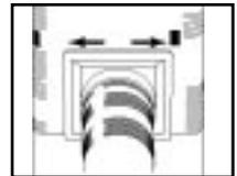
5. Push nozzle onto small connector end of vent duct pipe.
