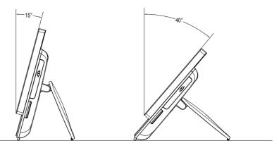
Use the stand to position the display to your preference. It can be rotated between 15° and 40° from the vertical.
