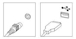
1.5.3 Connect the mouse cable to the appropriate mouse connector (USB connector).
