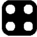
The HOT surface indicator lights on the cooktop surface will glow when their corresponding surface elements are turned on. The HOT surface indicator lights will continue to glow as long as the elements are too hot to touch, even after they are turned off.
