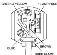
Upon completion there must be no cut, or stray strands of wire present and the cord clamp must be secure over the outer sheath.
