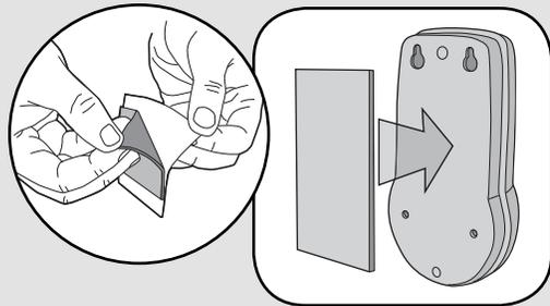
Peel off white paper from mounting tape. Firmly press mounting tape on back of doorbell.
