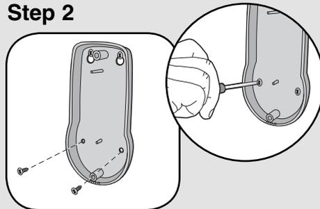
Put the remaining silver screws into the bottom holes of doorbell. Tighten screws.
