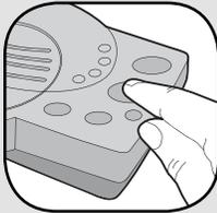
**Channel Button:** Press the Channel button to set intercom to one of four secure channels or the paging channel. The default channel for the intercom is the paging channel where all four channel lights are lit. An intercom on a channel can only hear an intercom on the same channel or on the paging channel.
