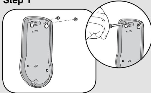
Mount doorbell with small silver screws. Screw the top two screws halfway into the mounting surface. Place back of doorbell over screws. Tighten screws.
