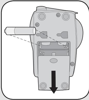
**Step 1:** Install 4 AA Alkaline batteries (not provided). (Lithium batteries recommended for colder environments.)
