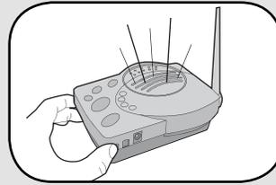
Press the Learn button on the new intercom until a beep is heard. Within 10 seconds put the second intercom into Learn Mode (refer to table below).
