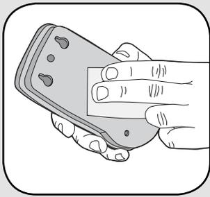
Clean back of doorbell and mounting surface using the alcohol wipe.
