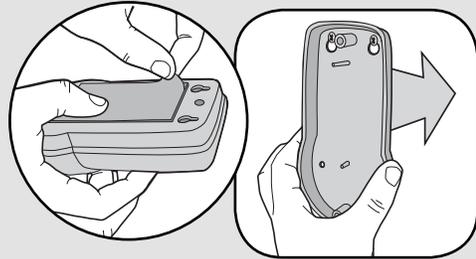
Peel paper from mounting tape. Firmly press doorbell onto mounting surface.
