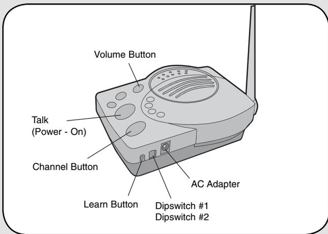
**On/Off:** To turn intercom ON, press any button. To turn intercom OFF, hold down the Volume button for 5 seconds.
