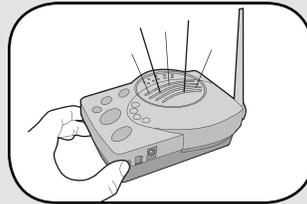
Press the Learn button on the new intercom until a beep is heard. Within 10 seconds put any networked intercom into Learn Mode (refer to table below).
