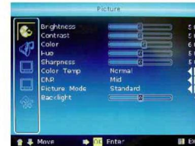
To display the OSD main menu, press the SYS MENU key on the remote control. Use the ◀ / ▶ keys to highlight the desired OSD Main Menu.
