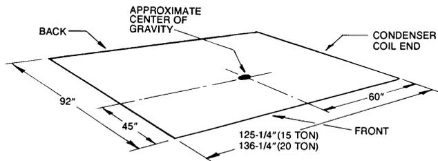
**FIGURE 2: CENTER OF GRAVITY**
