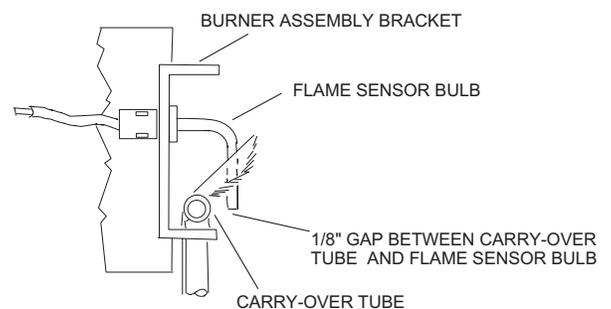
**FIGURE 17 : PROPER FLAME ADJUSTMENT**
