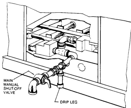
**FIGURE 6 : EXTERNAL SUPPLY CONNECTION EXTERNAL SHUT-OFF**
