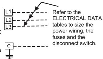
FIGURE 5 : TYPICAL FIELD WIRING
