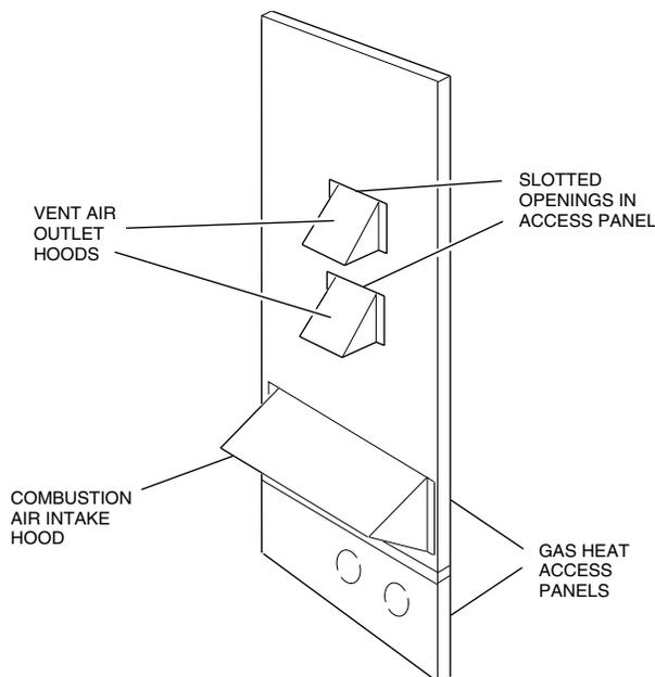
**FIGURE 8 : VENT AND COMBUSTION AIR HOODS**
