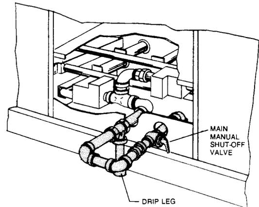
**FIGURE 7 : BOTTOM SUPPLY CONNECTION EXTERNAL SHUT-OFF**
