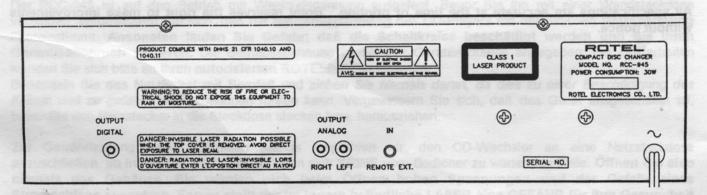
Please refer to this drawing which shows the analog, digital and external remote connections on the rear panel of the RCC 945.
