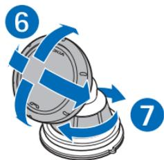
To detach the speakerphone from the mounting device, rotate it anticlockwise.
