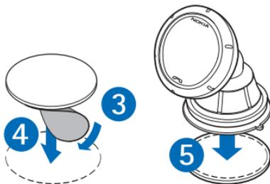
4. Peel off the protective sheet from the other side of the pad, and press the suction cup on the mounting device against the pad (5).
