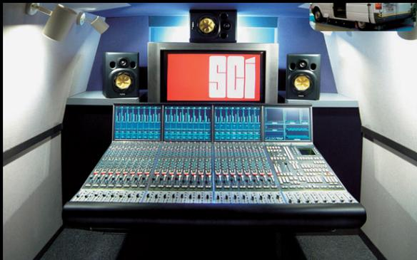
With demand for television programmes and DVD content on the increase, SCI felt it was time to upgrade its main vehicle so that it was better placed to cope with 5.1 surround sound productions. The C200 HD was an ideal console choice because it is very compact and can be tailored to fit into small spaces such as a mobile studio.
