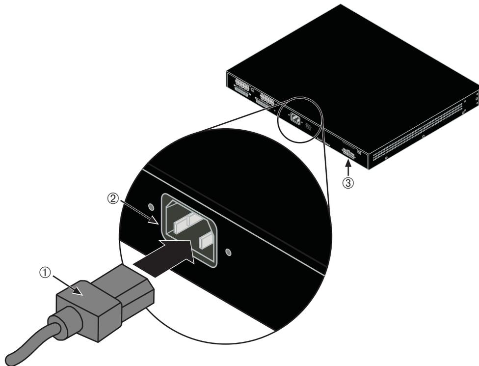
1 AC power cord 2 AC power connector 3 Connector for external redundant power supply
