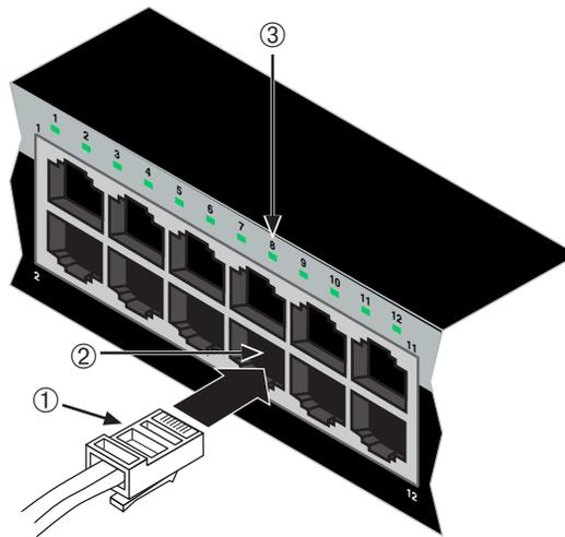
1 RJ45 connector                      2 Port 8                      3 Port 8 Link/Activity LED
