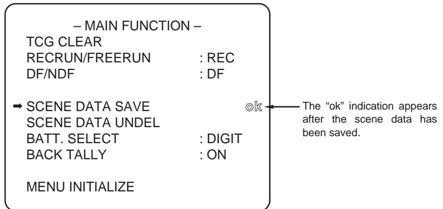
Use the ITEM button to align the arrow with the SCENE DATA SAVE position, and press the UP or DOWN button.
