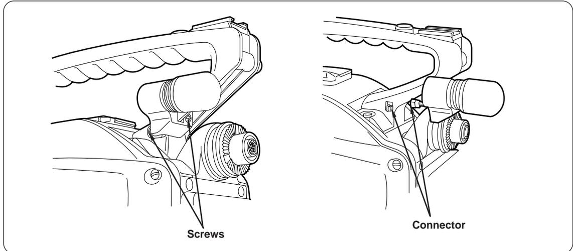
Remove the two screws to remove the connector and then remove the microphone.
