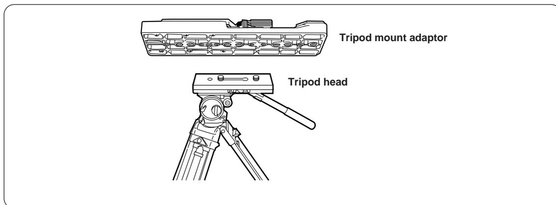
**NOTE:** Take the center of gravity of the unit and tripod mount adaptor into consideration when selecting the hole for the attachment. Also check that the diameter of the hole selected matches the diameter of the tripod head screw.
