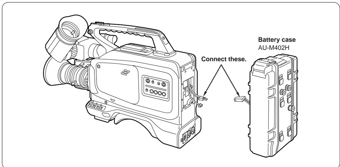
**3** Mount the AU-M402H battery case onto the unit using a screwdriver.
