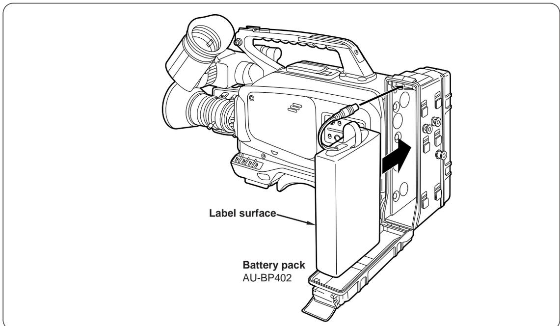
**CAUTION:** The unit's power must be turned off before the plug is connected or disconnected.
