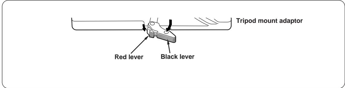
Move the black lever in the direction indicated by the arrow while holding down the red lever, and disengage the unit by sliding it toward you.
