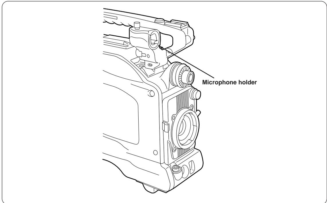
The microphone holder is attached by following the microphone removal procedure in reverse.
