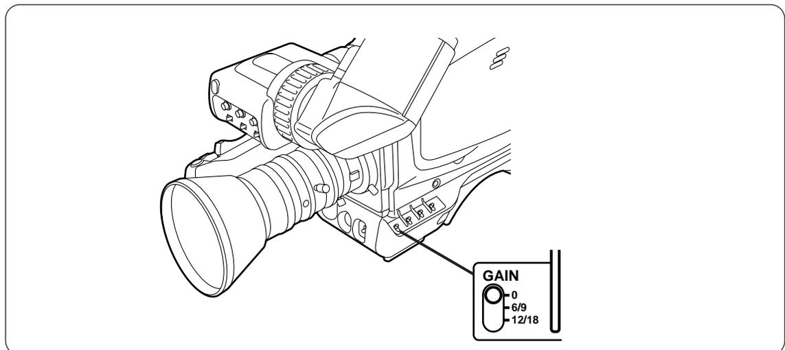
Gain settings of 0/6/12dB or 0/9/18dB are set on the menu item CAMERA SETTING menu screen for operation. (The 0/6/12dB settings were selected when the unit was shipped from the manufacturing plant.) For further details, refer to the menu items (on pages 48, 49 and 53).
