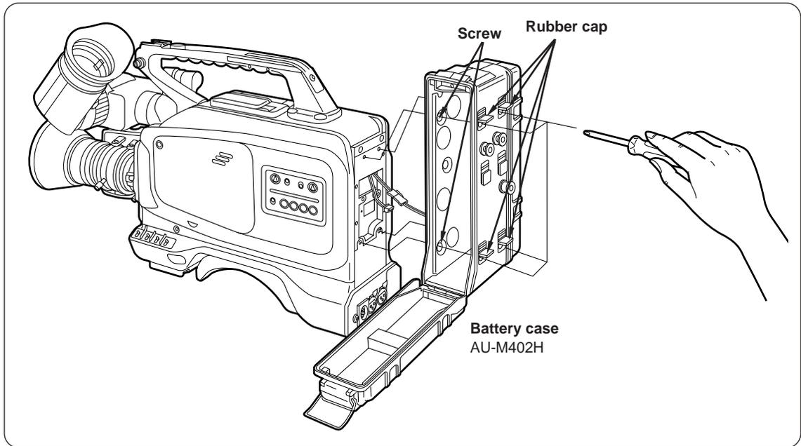
Holes with the screws recessed inside can be seen when the cover is opened and the rubber caps are lifted. Tighten up these screws using a screwdriver so that the battery case is mounted onto the unit. Tighten the screws up all the way.
