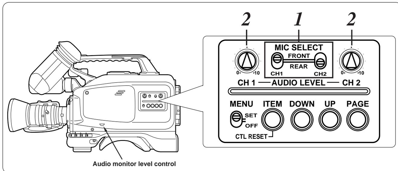
**1** Select the desired input signals using the audio input selector switches.
