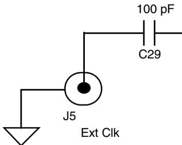
**Figure 2-4. J5 SMA Connection - (Optional) External Clock Input**
