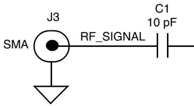
**Figure 2-3. J3 SMA Connection - Single TX/RX**
