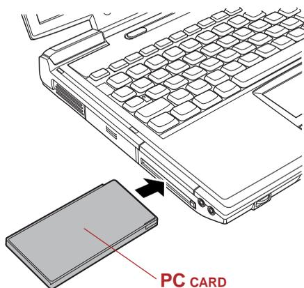
Figure 8-1 Installing the PC card
