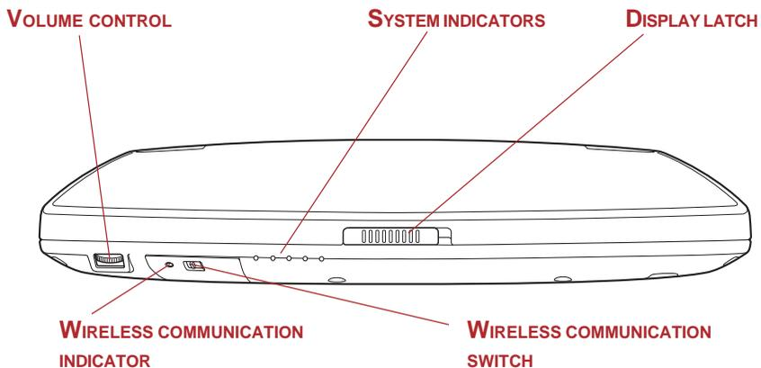
Figure 2-1 Front of the computer with display closed
