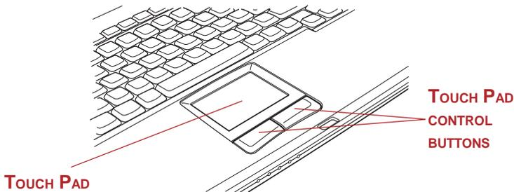
Figure 4-1 Touch Pad and Touch Pad control buttons
