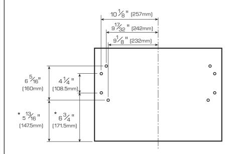
\* These dimensions are important to ensure a 1/4" (6mm) airflow gap.
