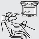
Installation of all TV monitors must be out of the drivers field of vision.
