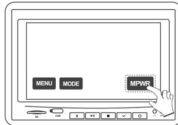
To power the off unit, press MPWR or PWR on the monitor; or press POWER button on the remote control.
