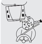
Do not mount the product where it will obstruct the deployment of the airbag or in an area where it would affect the driver's ability to control the vehicle. Also be careful to avoid mounting the product where it can become hazardous during sudden stops or in the event of an accident.
