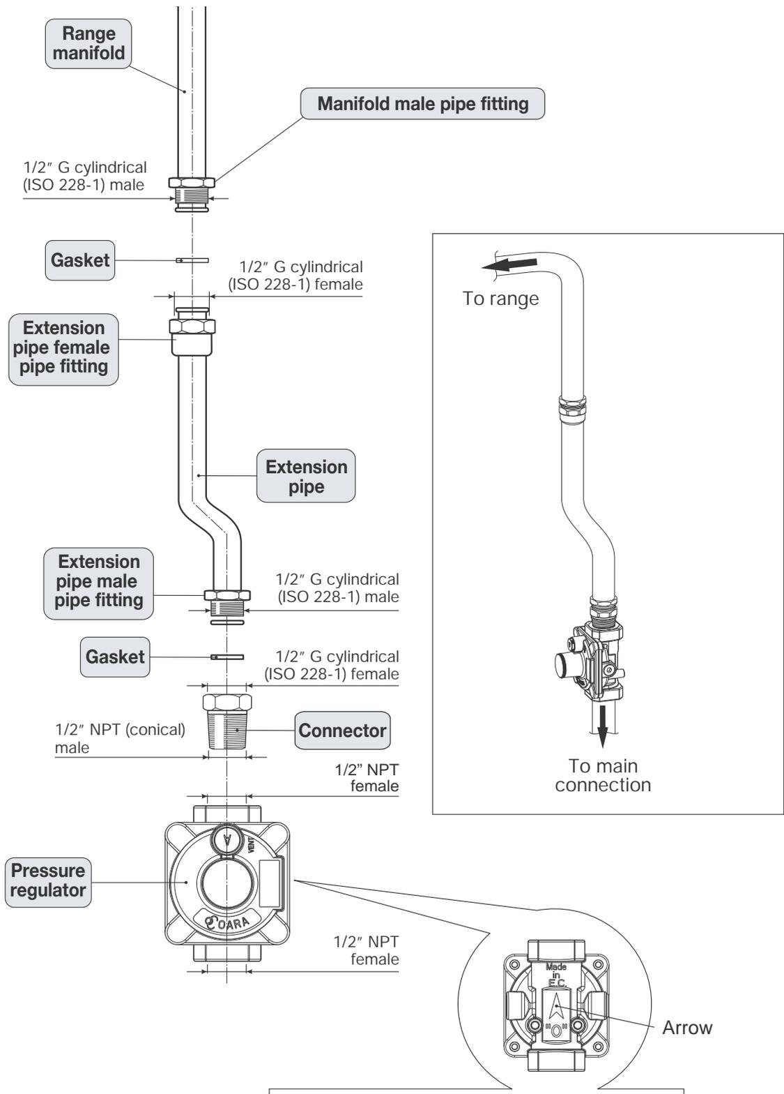
**WARNING: check the right positioning of the gas regulator. The arrow on the back of the gas regulator must be oriented toward the connector.**
