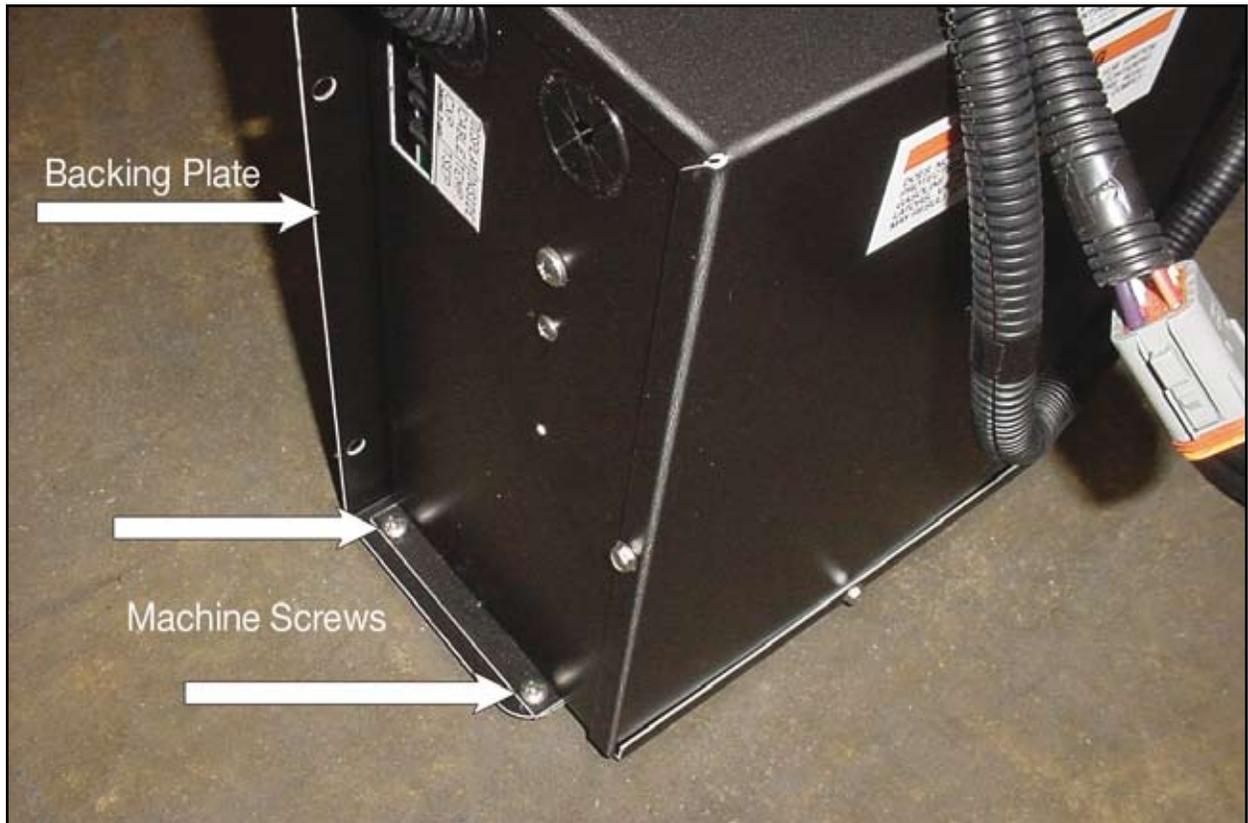
**Figure 3. Fastener location on Power Logic Box**
