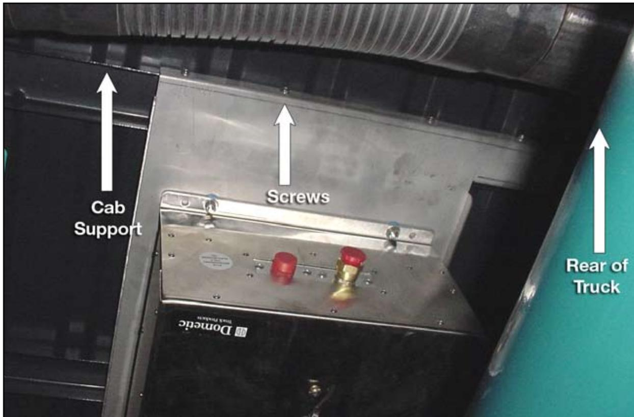
*Figure 16. Condenser installed on mounting plate.*
