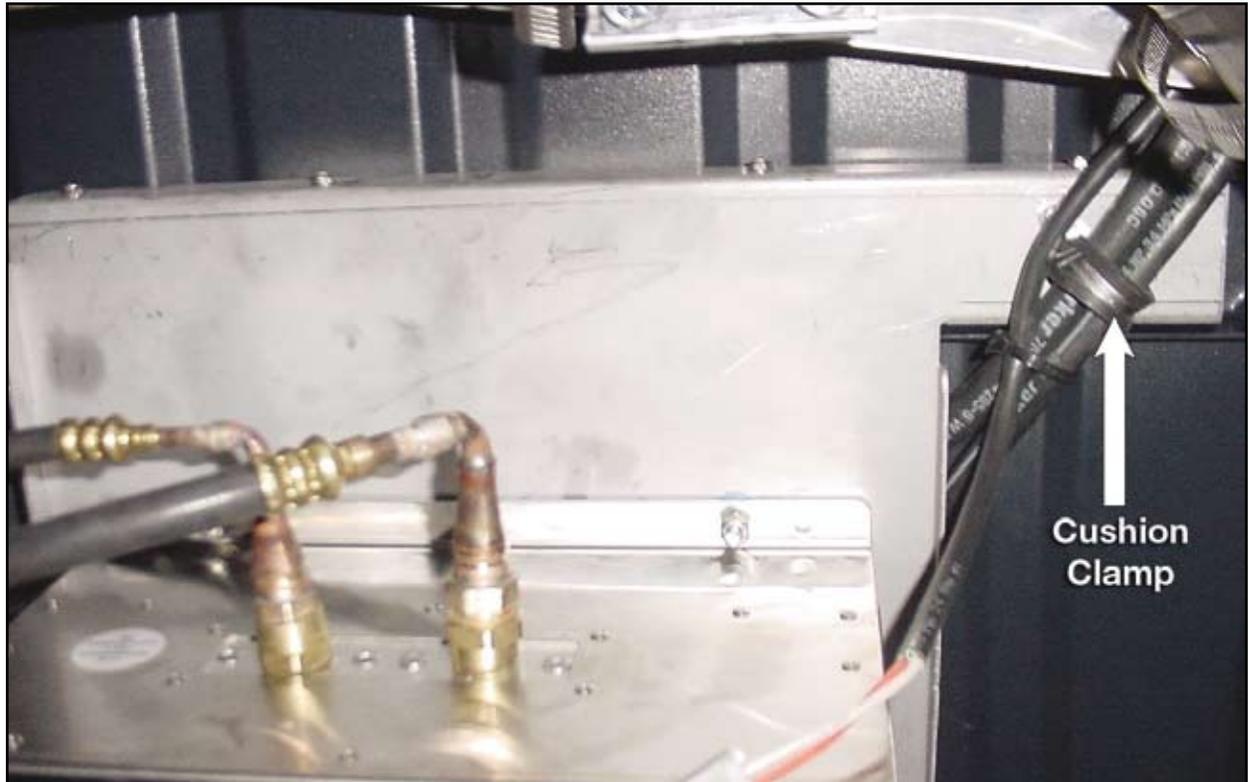
*Figure 17. Routing of refrigerant lines.*
