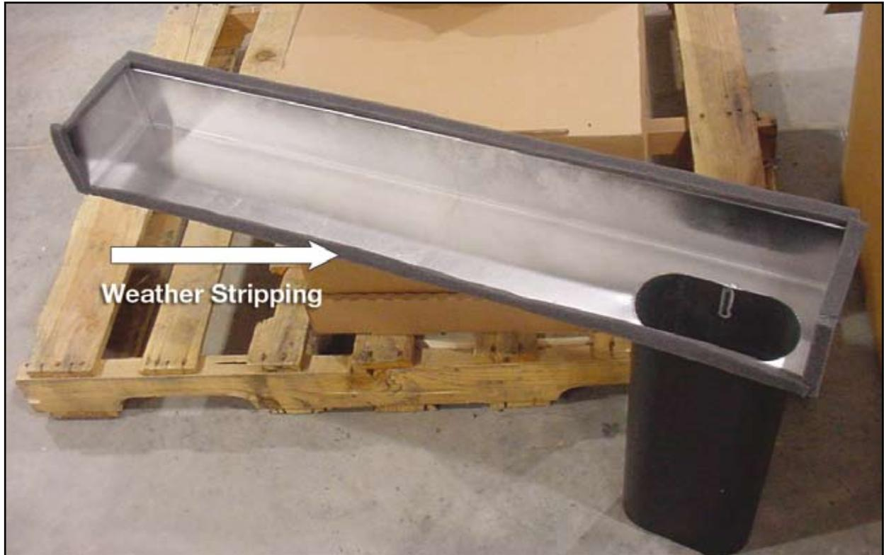
**Figure 9.** *Installing the weatherstripping on the custom plenum.*
