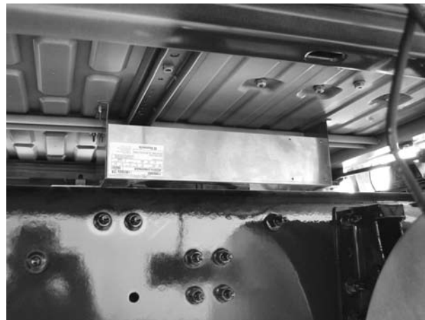
Figure 2a - Condensing unit mounted under truck
