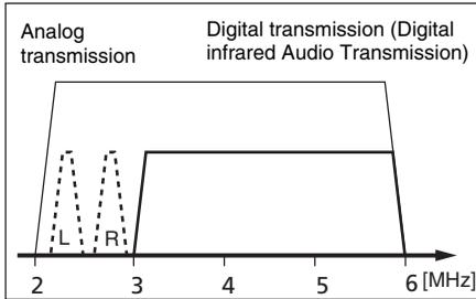
Fig. 1 Signal spectrum for digital infrared audio transmission
