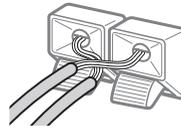
After connecting all the components, speakers, and AC power cord (mains lead), output a test tone to check that all the speakers are connected correctly. For details on outputting a test tone, see page 85. If no sound is heard from a speaker while outputting a test tone, or a test tone is output from a speaker other than the one currently displayed on the Setup Display, the speaker may be short-circuited. If this happens, check the speaker connection again.
