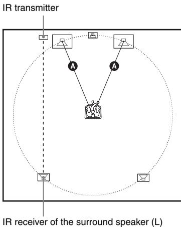
The following diagram indicates the infrared transmission area (the range that the infrared rays can reach).
