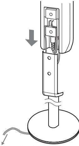
Adjust the length of the speaker cord (and the IR receiver cord).
