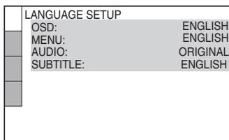
**4** Press **↑/↓** to select the setup item from the displayed list: **[LANGUAGE SETUP]**, **[SCREEN SETUP]**, **[CUSTOM SETUP]**, or **[SPEAKER SETUP]**. Then press **+**.
