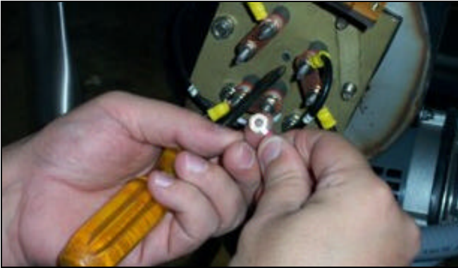
Fitting the jumper into the mounting cup.
