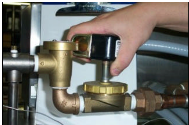
Removing the coil
