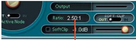
If we select the E node, the ratio in our example is displayed as 2.50:1. (For signals above the threshold, a 2.5 dB change in input level will yield 1 dB change in the output level.)
