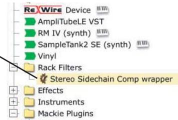
8. In the rack filter details area, set the input destinations of track 5 to be the left and right inputs to the compressor (this is the default setting, but check it anyway).
