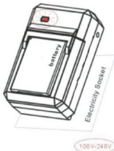
Plug your charger into an available electricity socket. When it is plugged in with a battery inserted, a red light will turn on to indicate the battery is charging.
