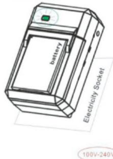
When your battery is fully charged, the light on the charger will turn green.
