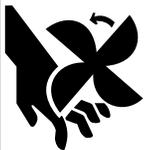
1.d. Keep all equipment safety guards, covers and devices in position and in good repair. Keep hands, hair, clothing and tools away from V-belts, gears, fans and all other moving parts when starting, operating or repairing equipment.
