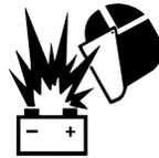
**GASES FROM BATTERY** can explode.
