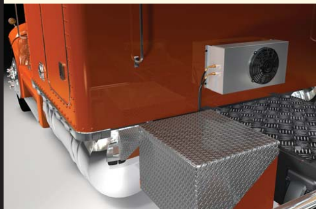
Split system external condenser.
