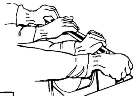
4. Carefully insert downdraft vent into countertop cutout. Two people are recommended to support the weight of the downdraft vent during lifting. Check that downdraft vent is parallel to side of cutout and that mounting brackets overlap countertop.
