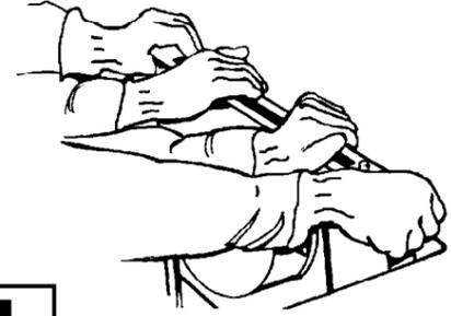
**4.** Carefully insert downdraft vent into countertop cutout. Two people are recommended to support the weight of the downdraft vent during lifting. Check that downdraft vent is parallel to side of cutout and that mounting brackets rest gently on countertop.
