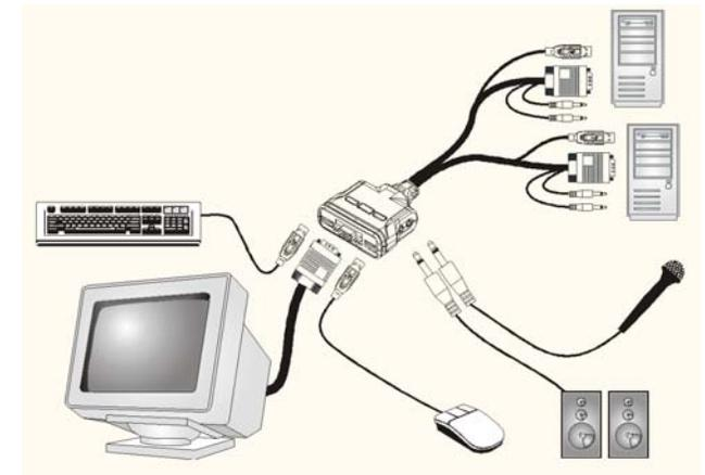
**Step 6** Connect each of the built-in KVM cables to a computer's video and usb ports. You can also connect the cables to the computer's audio and microphone ports.
