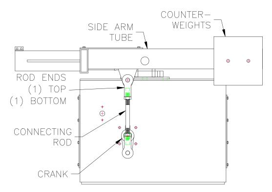
5) Manually rotate the barrier into its fully closed to traffic position.
