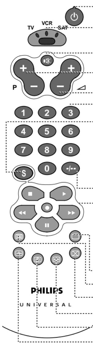
**Power** switches TV/VCR/SAT on and off
