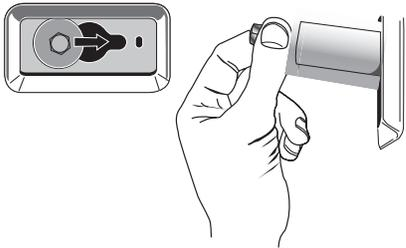
3. Once all 4 bolts are removed, discard the bolts and spacers. Then pull the power cord through the opening of the rear panel and close the hole with the attached cap.
