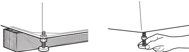
If the washer is against a wall, move the washer out slightly before tipping back. If the washer is not level, first prop the front with a wooden block and adjust the front feet height moving the hexagonal plastic part as necessary. Repeat to adjust back feet.
