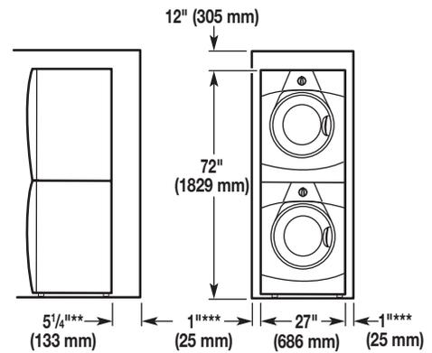
\*Min. top and bottom air openings for closet door.
