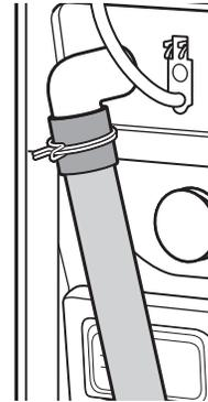
4. Washer drain system can be installed using a floor drain, wall standpipe, floor standpipe, or laundry tub.
