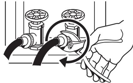
**NOTE:** Do not overtighten. Damage to the coupling or water faucet can result. Both faucets must be turned on for the washer to work properly.
