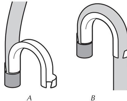
A. Snap either end of the drain hose form to the drain hose at the point where the corrugation begins.
