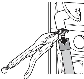
2. Slide drain hose onto washer connection.
