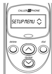
1. Press and hold the up arrow button then press and hold the down arrow button. Continue to hold both buttons for 3 seconds. **SETUP MENU ^ v** appears.
