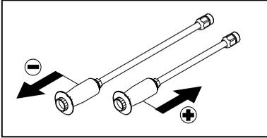
After pulling backwards to high pressure, turn wand left or right to change the spray pattern between point jet and flat jet.
