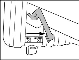
After engine has warmed and idles smoothly, **move CHOKE lever to the RUN position as indicated.**
